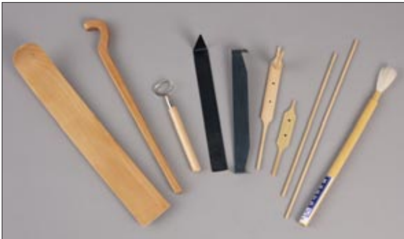
▼ Tools for porcelain production 2020-2022 made from Japanese oak, aluminium, steel, bamboo, and sheep hair.
