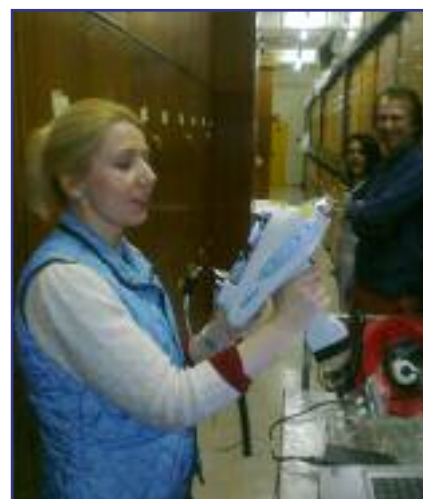
▲ Amelie Drewden using the X-ray Fluorescence Analysis (XFA) machine to analyse possible pesticide residues on biological specimens
