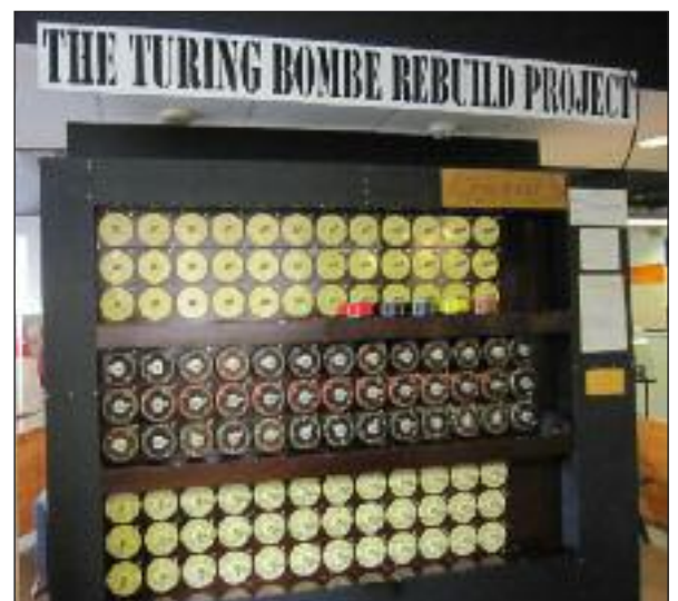
▼ Turing Bombe Rebuild Project - this electromechanical machine was designed by Turing for codebreaking. Gordon Welchman improved on this machine. 200 Bombes were made and used in the war.
