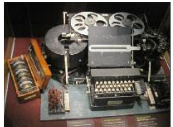
▲ Typex machine - this deciphered and printed out code from the German encyphering machine Enigma
