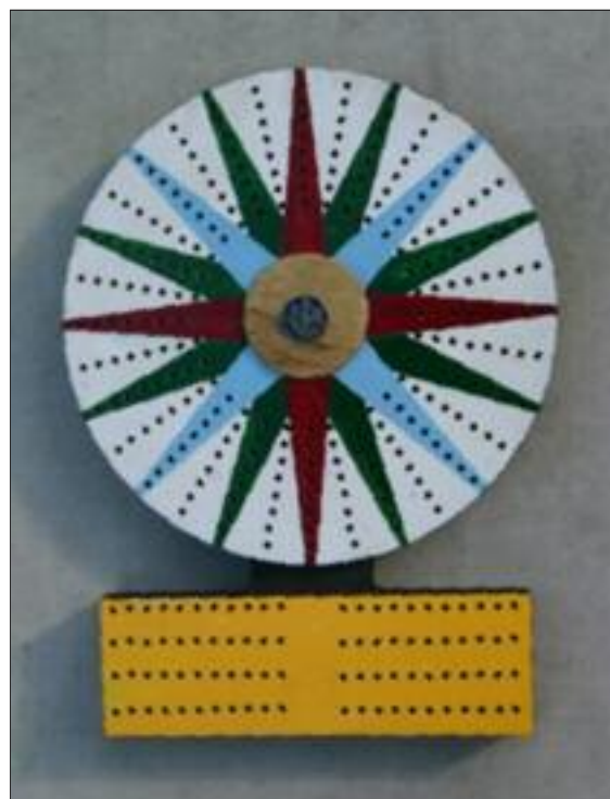
▲ The traverse board was a memory aid used in dead reckoning navigation to record with pegs and cord the speed and direction sailed during a watch
