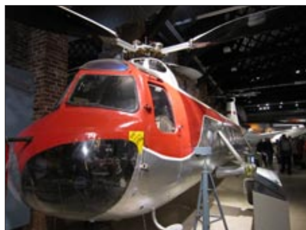
▲ Bristol Type 173 Helicopter Prototype – first registered 1948 – powered by 2 Alvis Leonides radial piston engines
