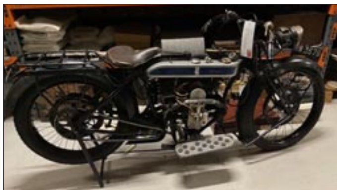
▲ A 2-cylinder 350cc Douglas CW25 motorcycle built by Douglas Motors Ltd in Kingswood in 1925. Square section petrol tanks were popular in the 1920s.
