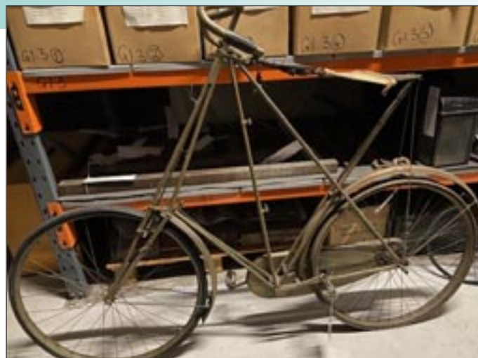
▲ A Dursley Pedersen gentleman's chain-driven cantilever frame safety bicycle, made in Dursley in 1906.
