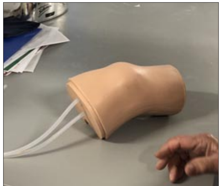
▼ Completed ultra-sound knee which has been over-moulded with silicone ready to be tested
