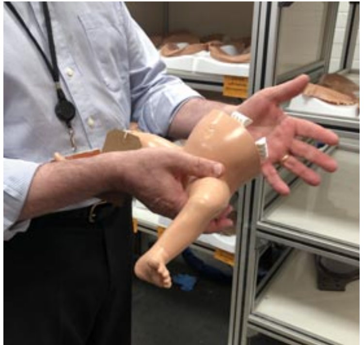
▲ Lower moulded section of an infant hip trainer waiting to be transferred into the assembly department
