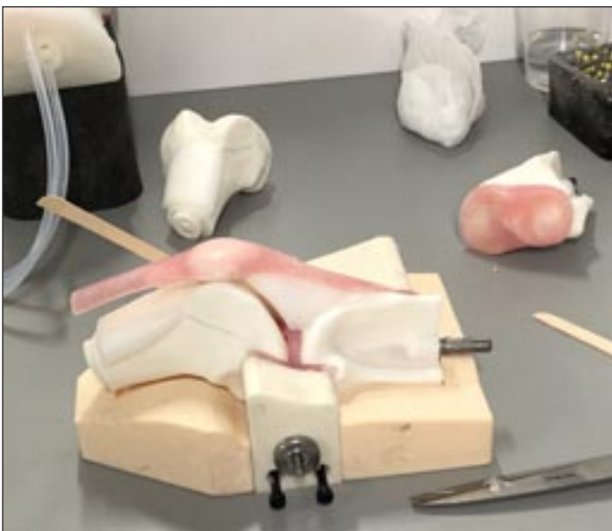
▼ First stage of producing an ultra-sound knee: the bones placed onto an assembly jig in the assembly department
